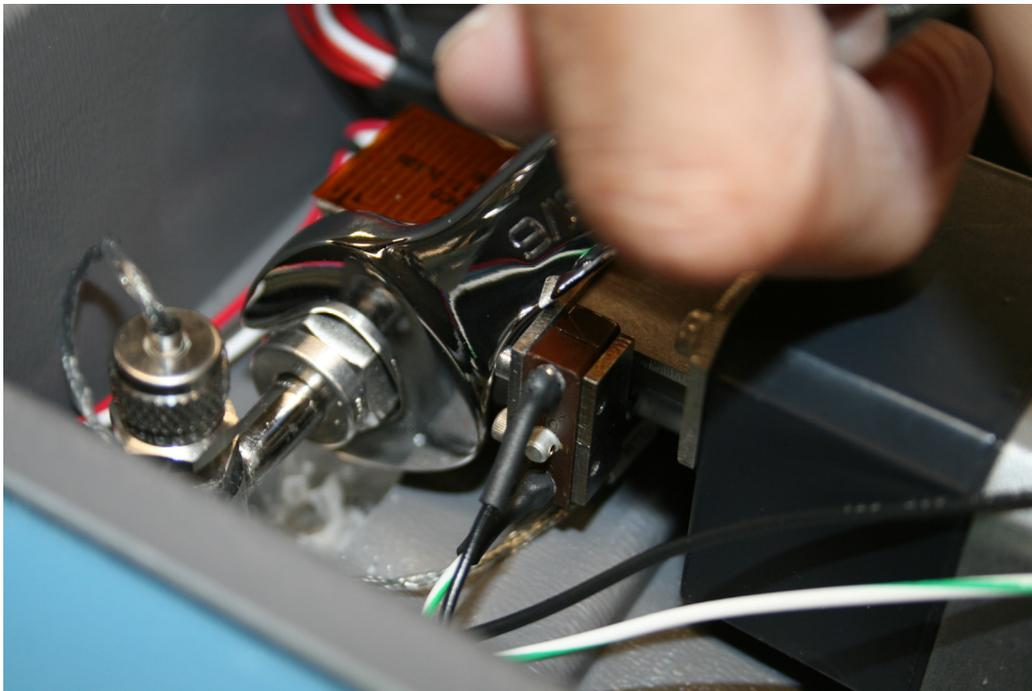
7. Rotate the valve motor 90° up.
